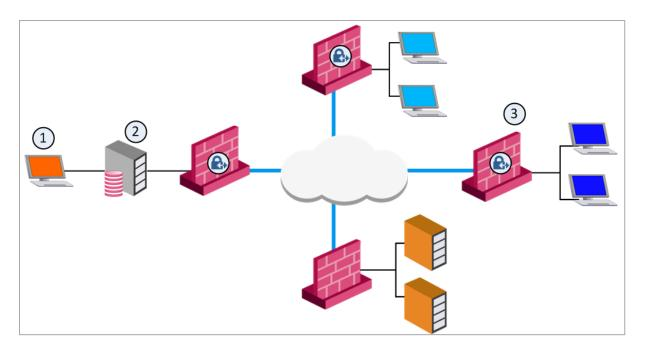
SIC is initialized between Security Gateways (3) (local and remote), and the Security Management Server (2). The Security Management Server then gets status data from the Software Blades with the **AMON** (Application Monitoring) protocol. SmartView Monitor (1) gets the data from the Security Management Server.
